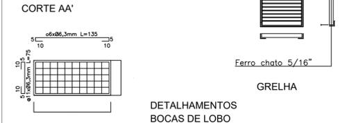
4 DETALHAMENTO BOCAS DE LOBO SEM ESCALA
